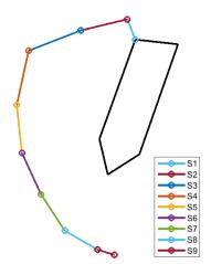
Figure 1: Segmentation of the blade (names sequential from stump to toe)
